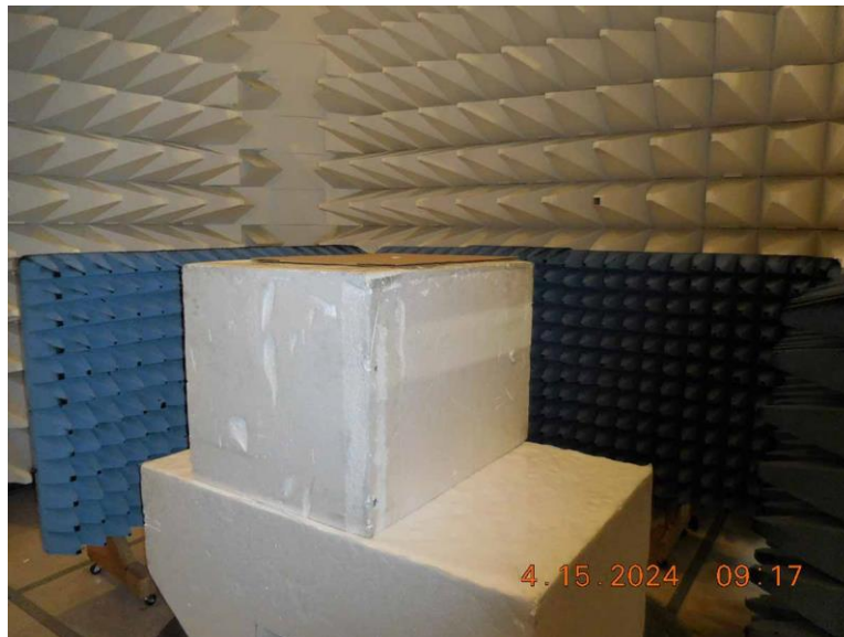
Above 1GHz, Overall Test Setup
