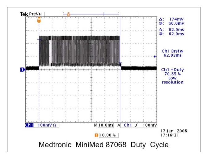
Note: The video output of a spectrum analyzer was monitored with the O'scope to capture and measure the duty cycle of the transmission burst. Several captures were made to determine the range of duty cycle values, and the worst case measured was saved. Captured O'scope display, showing a 70.85% duty cycle within a 62ms burst. This equates to a total on-time of 43.9ms during a 100ms window, which calculates out to a duty cycle correction factor of -7.1 dB.
