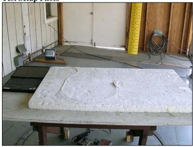
**Test Conditions:** The EUT is placed on the wooden table with 10 cm of Styrofoam. The EUT is connected to the USB port of a support laptop via a 2 meter, shielded USB cable. Frequency = 916.5 MHz. The laptop is running test routines to exercise the EUT. The EUT transmits and receives data packets to a support receiver in the vicinity. The emissions profile of three orthogonal orientations was investigated. Data set represents worst case emission: flat.
