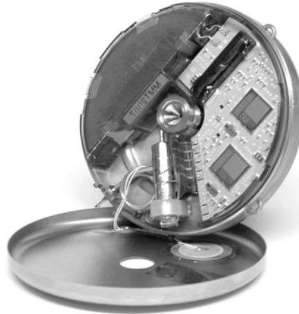
Figure 2: Interior of the Implantable Insulin Pump
