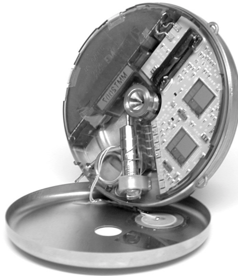
Figure 3: Interior of the Implantable Insulin Pump
