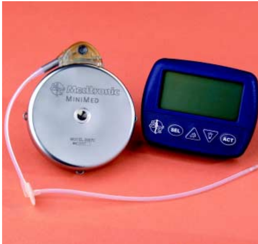
Figure 1: Personal Pump Communicator (PPC) and Implantable Insulin Pump
