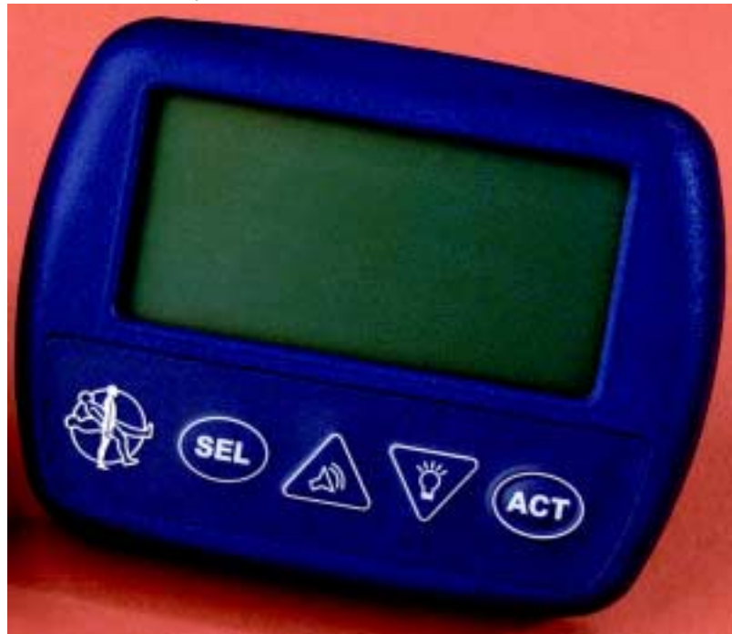
Figure 5: Personal Pump Communicator (PPC)
