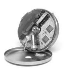
Figure 2: Interior of the Implantable Insulin Pump
