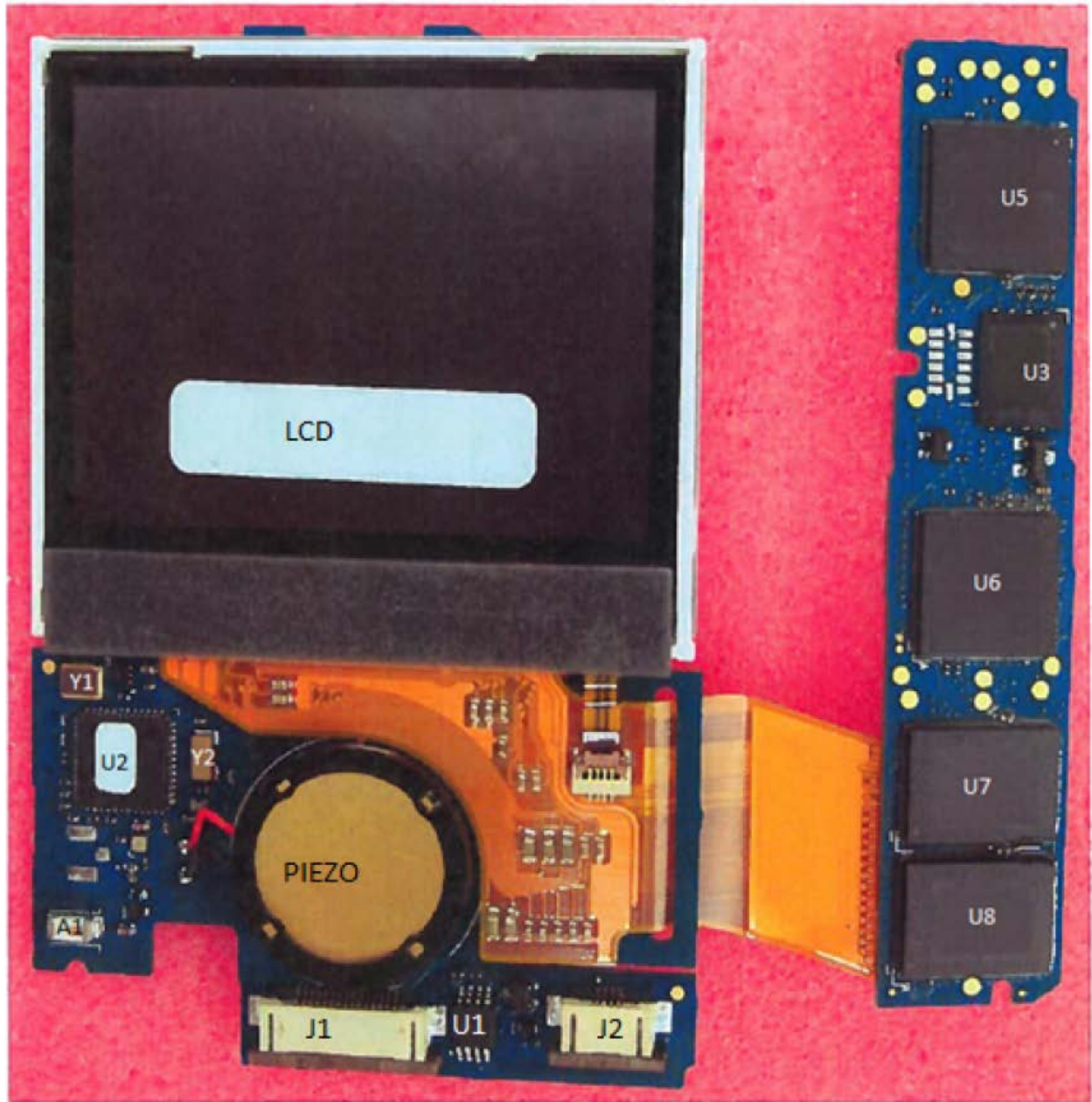
Minimed 620G PCBA Stack Opened: Top View
