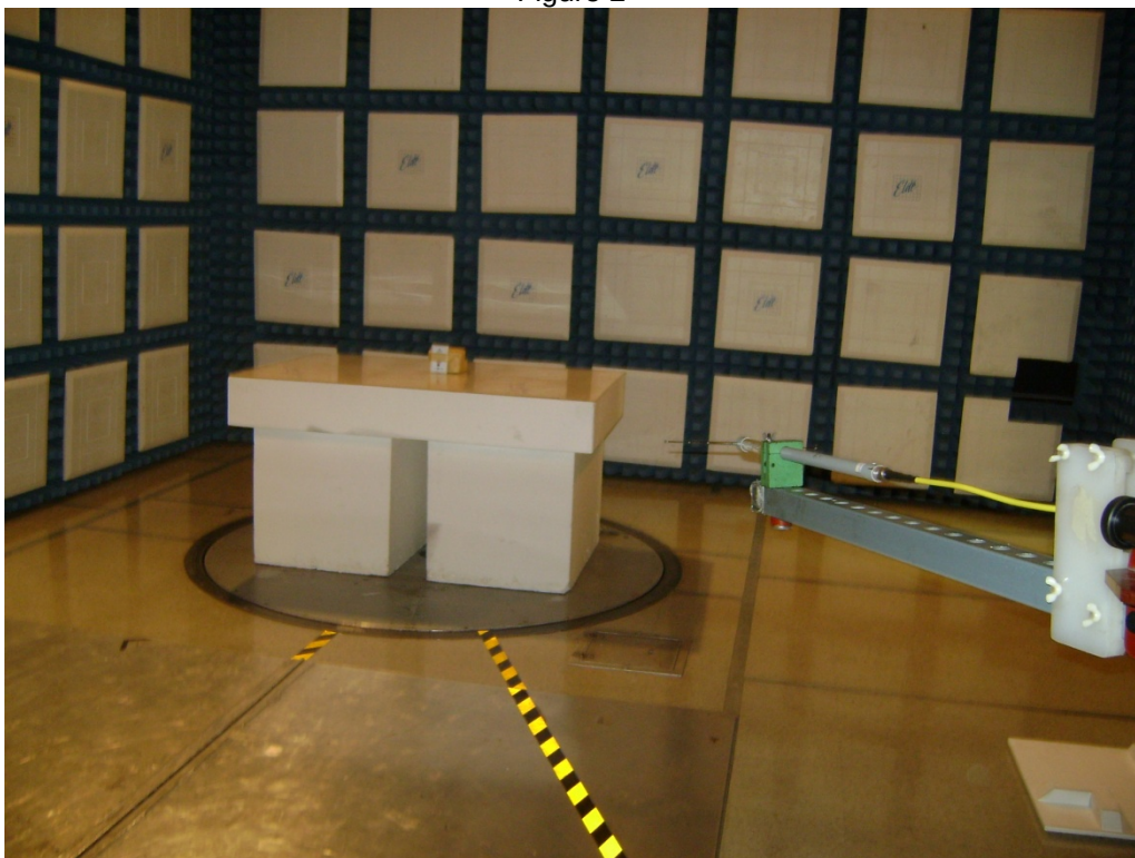
Test Setup for Radiated Emissions – Horizontal Polarity
