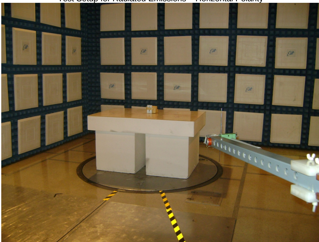
Test Setup for Radiated Emissions – Vertical Polarity
