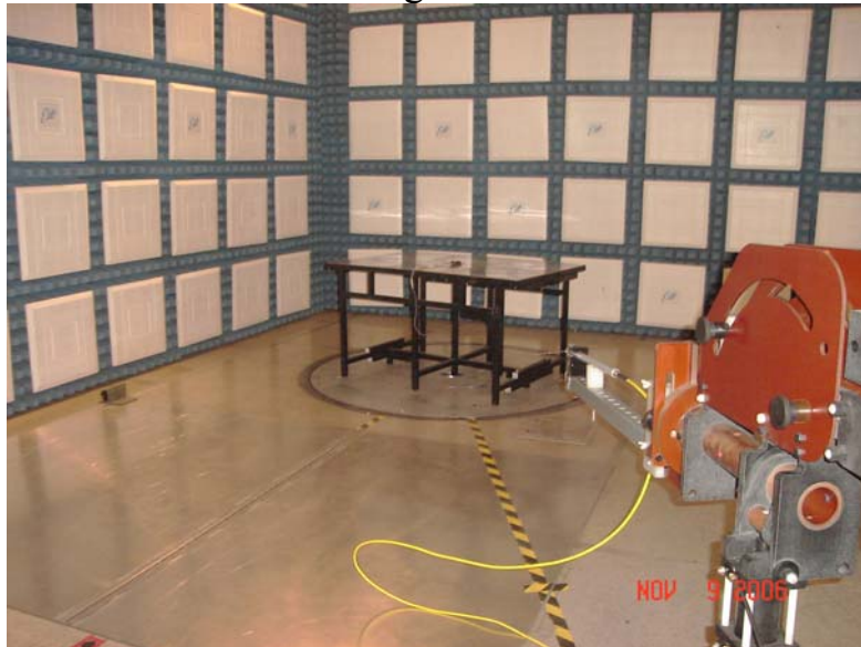
Test Set-up for Radiated Emissions Horizontal Polarity
