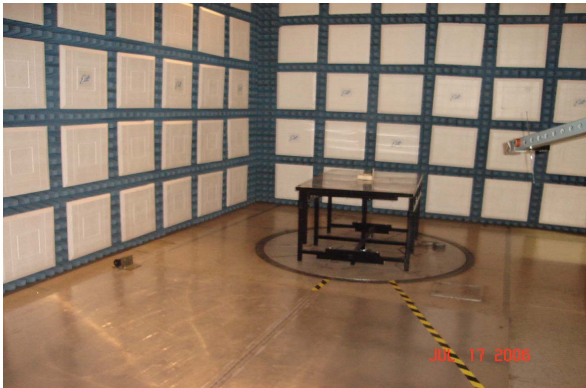
Test Set-up for Radiated Emissions Vertical Polarity
