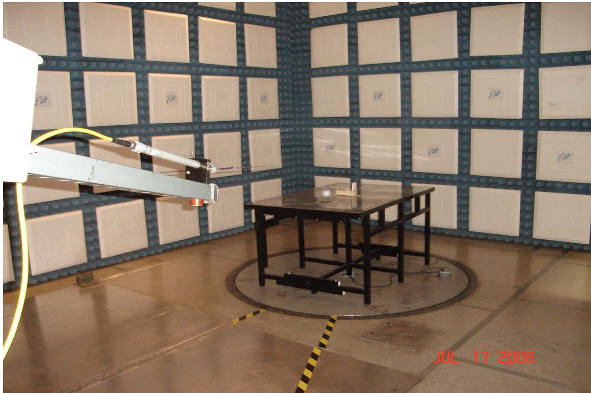
Test Set-up for Radiated Emissions Horizontal Polarity
