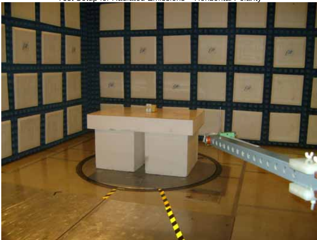
Test Setup for Radiated Emissions – Vertical Polarity
