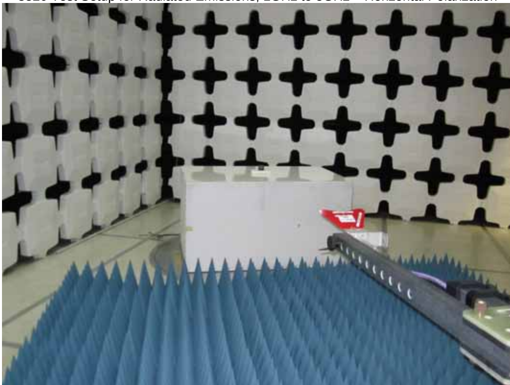
3520 Test Setup for Radiated Emissions, 1GHz to 5GHz – Vertical Polarization
