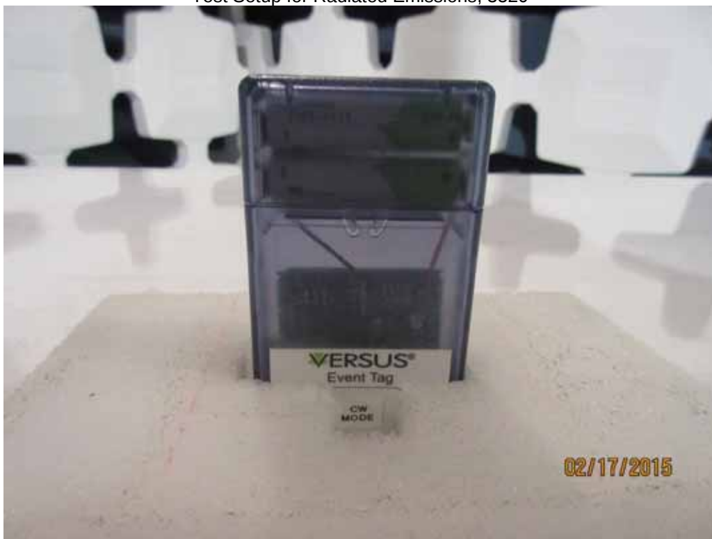
Test Setup for Radiated Emissions, 3522
