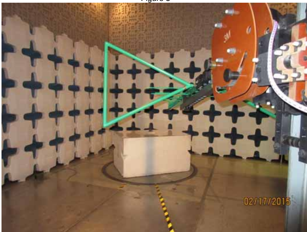
3522 Test Setup for Radiated Emissions, 30MHz to 1GHz – Horizontal Polarization
