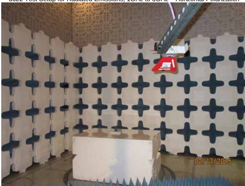
3522 Test Setup for Radiated Emissions, 1GHz to 5GHz – Vertical Polarization
