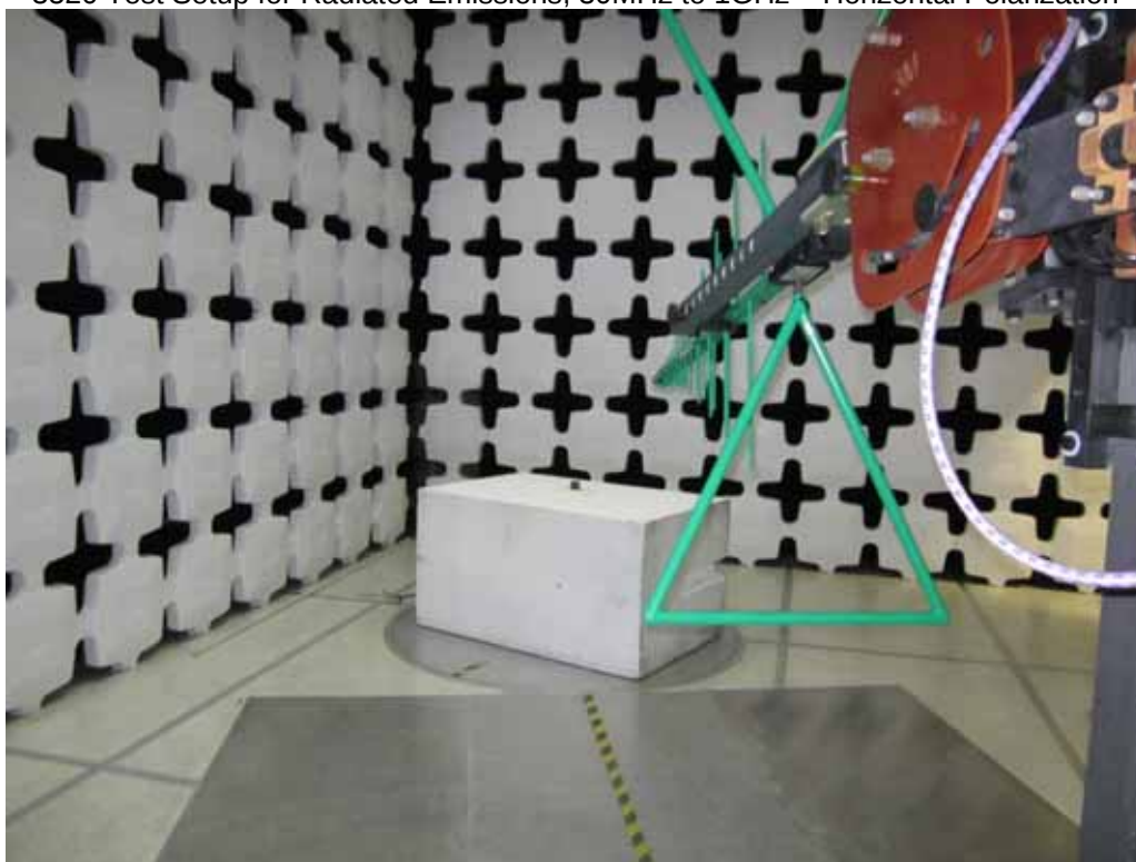
3520 Test Setup for Radiated Emissions, 30MHz to 1GHz – Vertical Polarization
