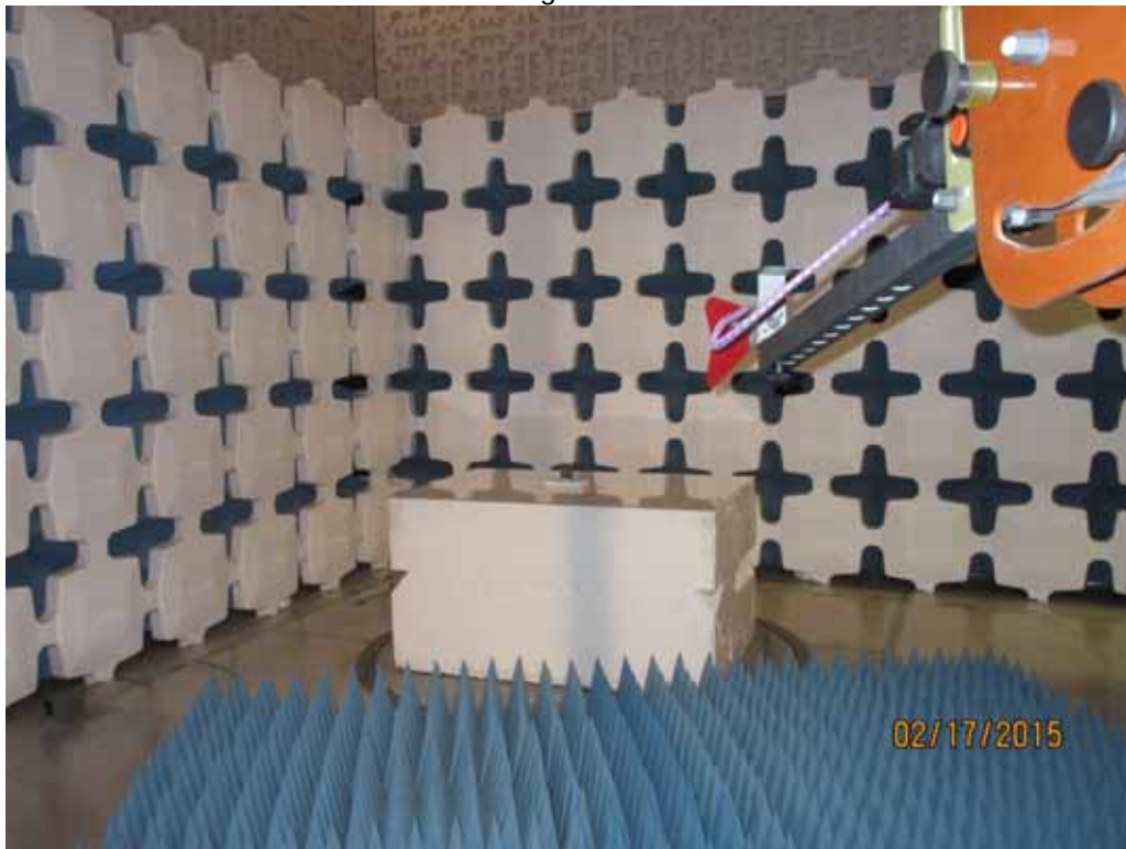
3522 Test Setup for Radiated Emissions, 1GHz to 5GHz – Horizontal Polarization
