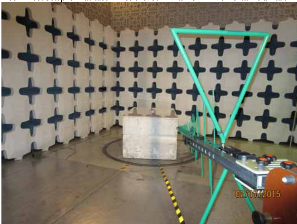
3522 Test Setup for Radiated Emissions, 30MHz to 1GHz – Vertical Polarization
