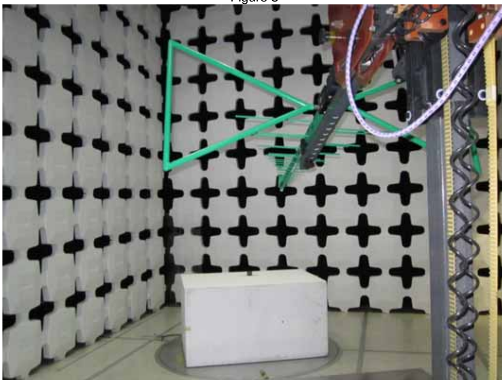
3520 Test Setup for Radiated Emissions, 30MHz to 1GHz – Horizontal Polarization
