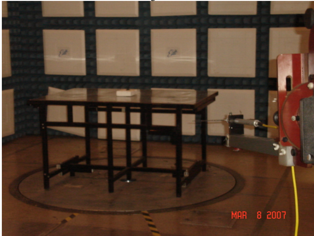
Test Setup for Radiated Emissions, 434MHz – Horizontal Polarity
