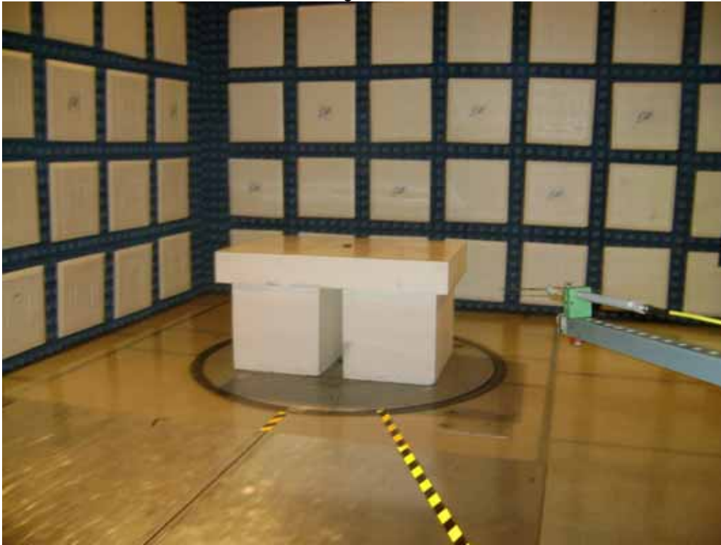
Test Setup for Radiated Emissions – Horizontal Polarity
