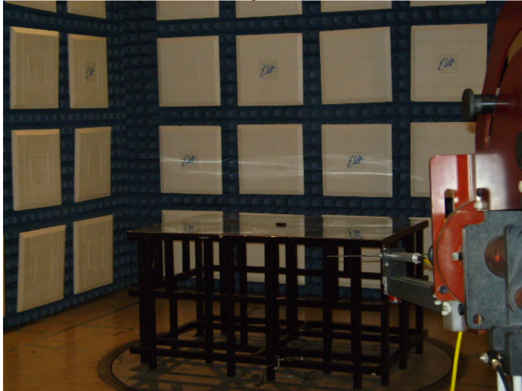
Test Set-up for Radiated Emissions – Horizontal Polarity
