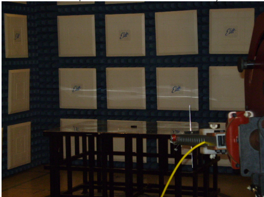
Test Set-up for Radiated Emissions – Vertical Polarity
