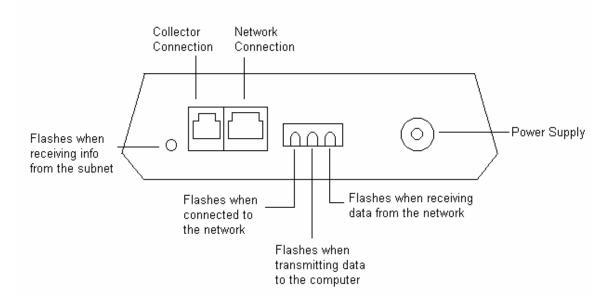
The LED indicator light on the Collector will blink every time it receives badge data from the sensors. If the LED blinks in a four or 5-blink pattern, this indicates that it is not communicating with the concentrator. If this is the case, there is a problem with either the network cable connection or the connection to the concentrator. If the LED blinks in a 3-blink pattern, this indicates a problem with the collector, and it should be sent to Versus Technology for repair.
