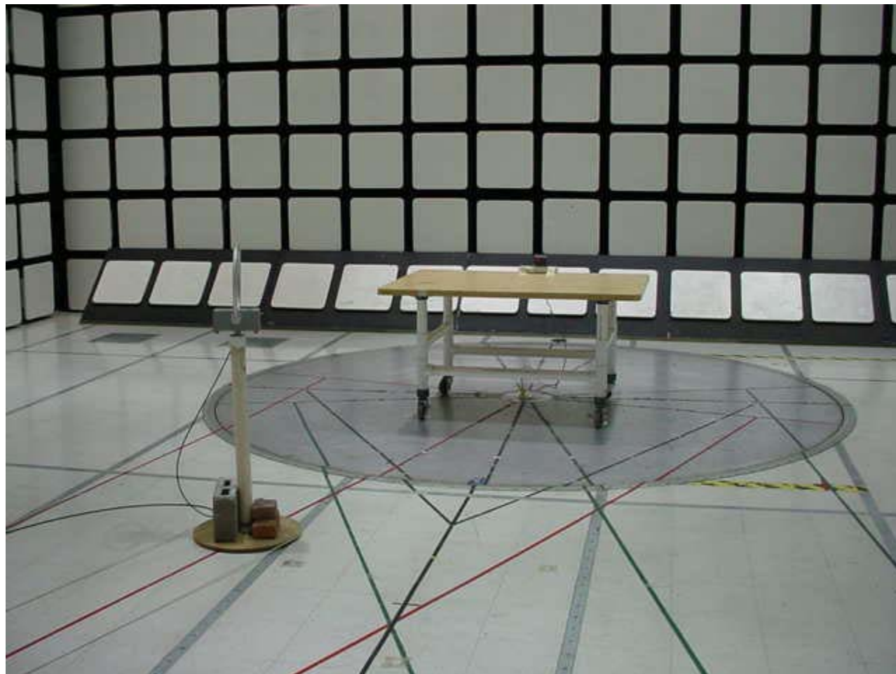
Radiated Emissions Test Setup (9k – 30MHz)
