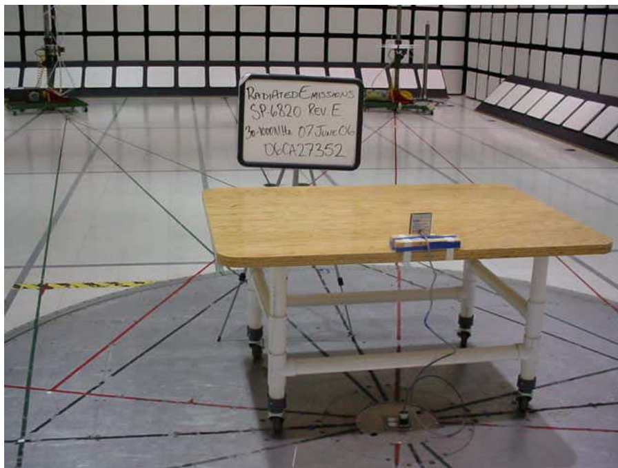
Radiated Emissions Test Setup (30 – 1000MHz)
