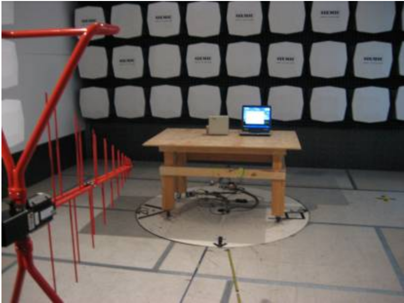
Radiated Emission Test Set-up Front View ( 0.3 - 1 GHz )
