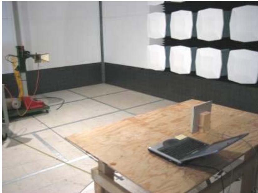
Radiated Emission Test Set-up Rear View (> 1 GHz)
