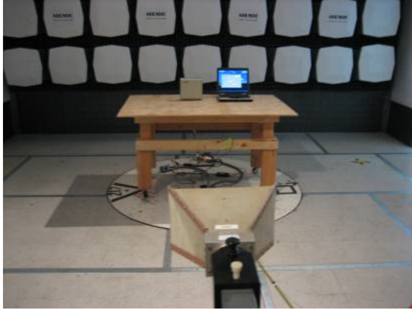
Radiated Emission Test Set-up Front View (> 1 GHz)
