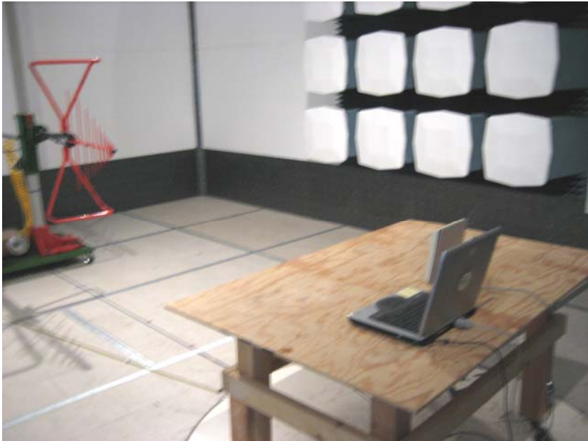
Radiated Emissions Test Set-up Rear View ( 0.3 - 1 GHz )
