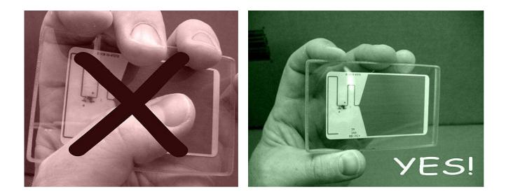
Body-blocking of the GMWS Glass-Mounted Windshield Tag, for use with AWID's LR-911 Long-Range Reader, can be eliminated by holding the glass rectangle as shown in the photograph above. This method of holding the tag keeps the hand behind the glass, away from the reader.
