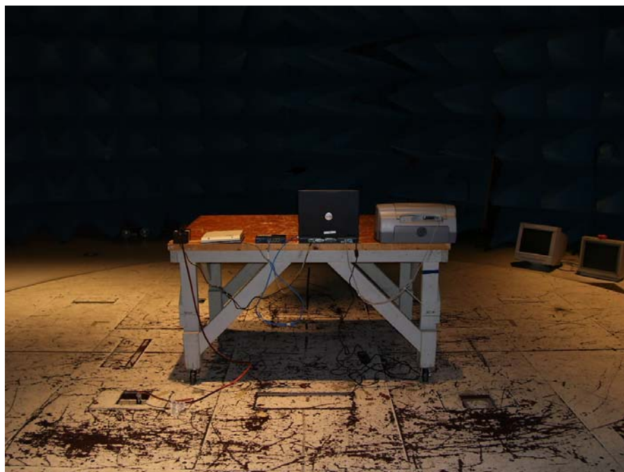
Photograph 7. Radiated Emission Test Setup 30 MHz - 1 GHz, Back View, LR911
