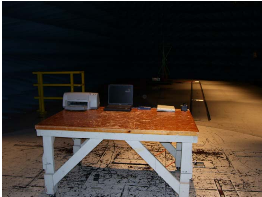
Photograph 6. Radiated Emission Test Setup 30 MHz - 1 GHz, Front View, LR911
