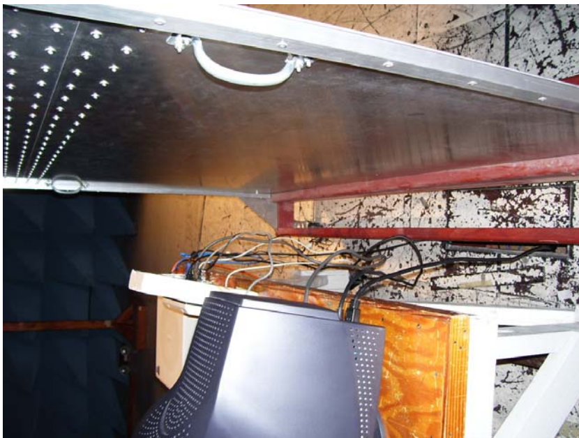
Photograph 13. Conducted Limits, Test Setup, Back View 2010-AR
