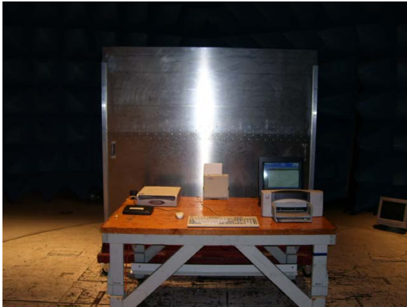
Photograph 12. Conducted Limits, Test Setup, Front View 2010-AR
