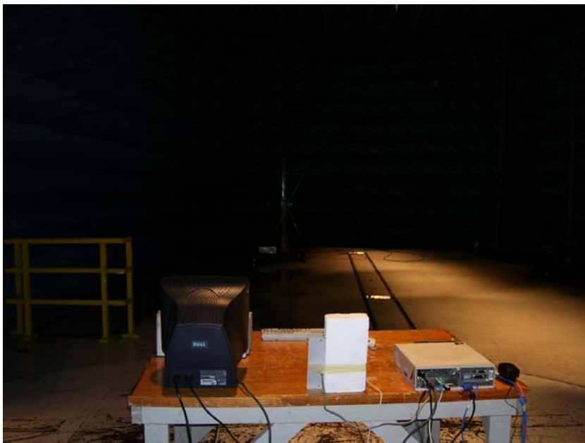
Photograph 9. Radiated Emission Test Setup 30 MHz - 1 GHz, Back View 2010-AR
