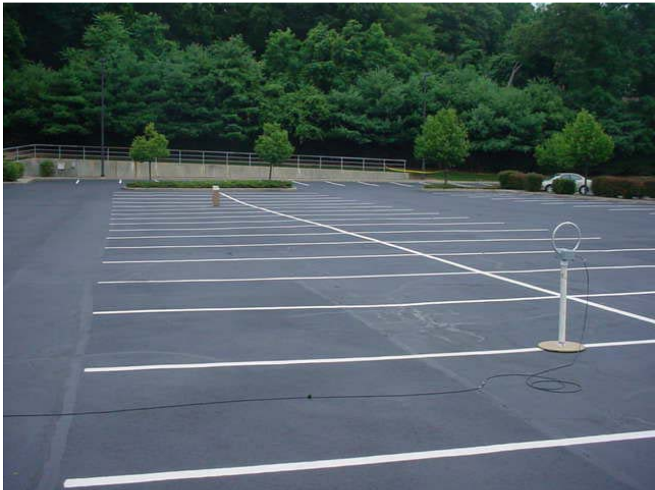
Radiated Emissions Test Setup – 30M Measurement
