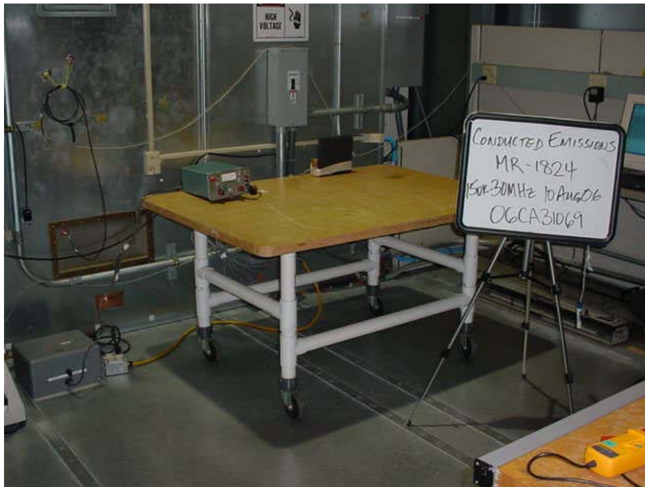
Conducted Emissions Test Setup (150kHz - 30MHz)
