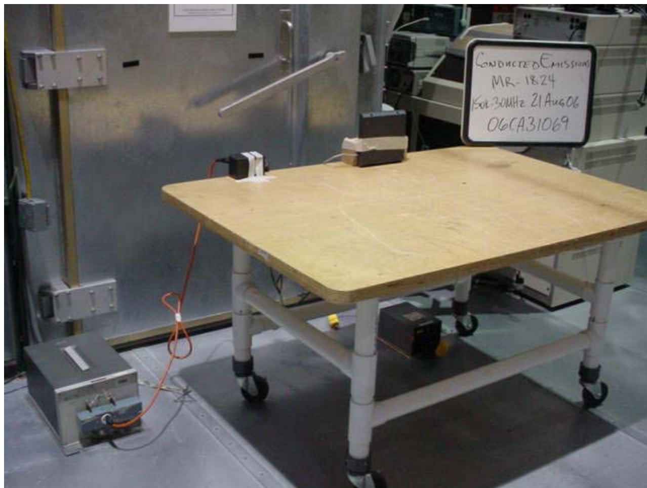
Conducted Emissions Test Setup (150kHz – 30MHz)
