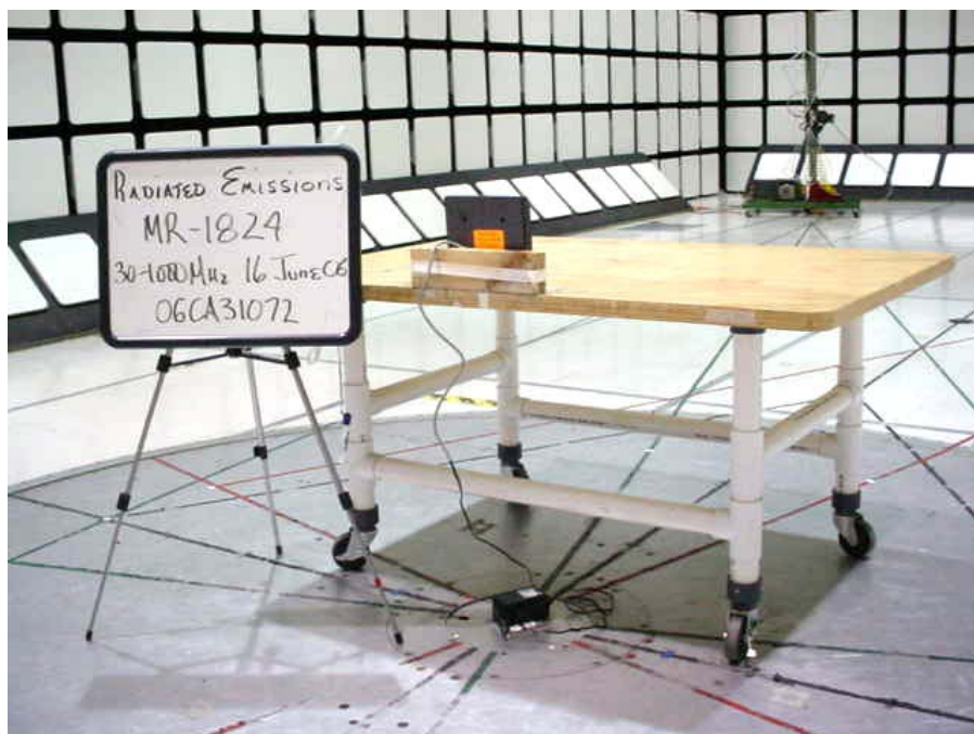
Radiated Emissions Test Setup 30 – 1000MHz
