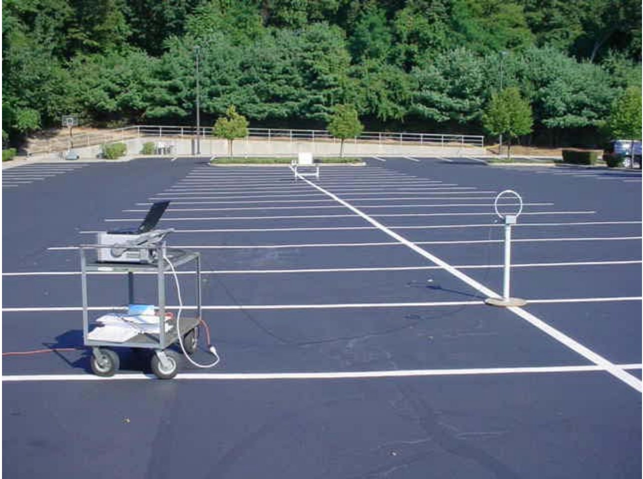
Radiated Emissions Test Setup (30M Measurement)
