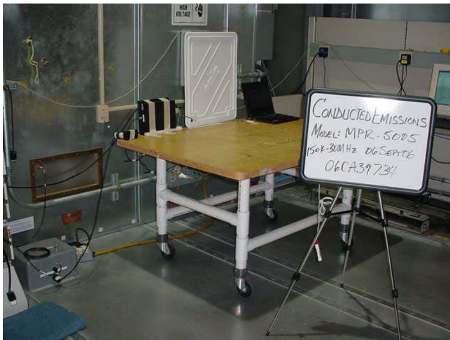
Conducted Emissions Test Setup (150kHz – 30MHz)
