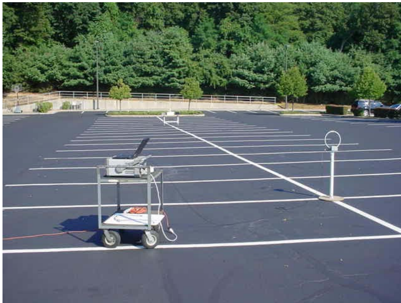
Radiated Emissions Test Setup (30M Measurement)
