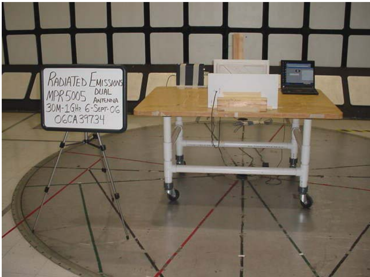
Radiated Emissions Test Setup (30-1000MHz)
