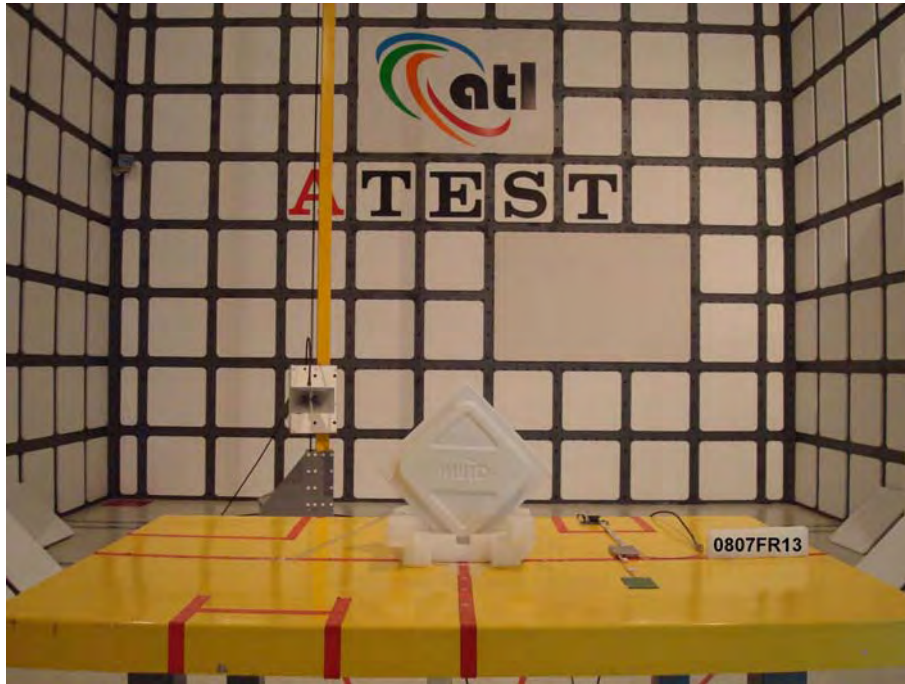
Figure 10. Front View of the Test Configuration _ EUT with Antenna (ANT-915CPS-A)
