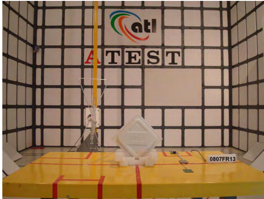
Figure 8. Front View of the Test Configuration _ EUT with Antenna (ANT-915CPS-A)
