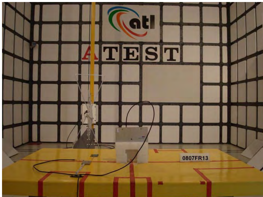
Figure 13. Rear View of the Test Configuration _ EUT with Antenna (ANT-2010CP)
