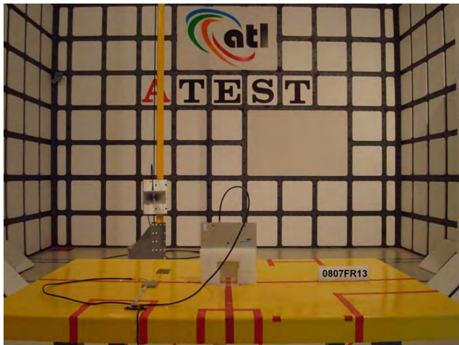
Figure 15. Rear View of the Test Configuration _ EUT with Antenna (ANT-2010CP)
