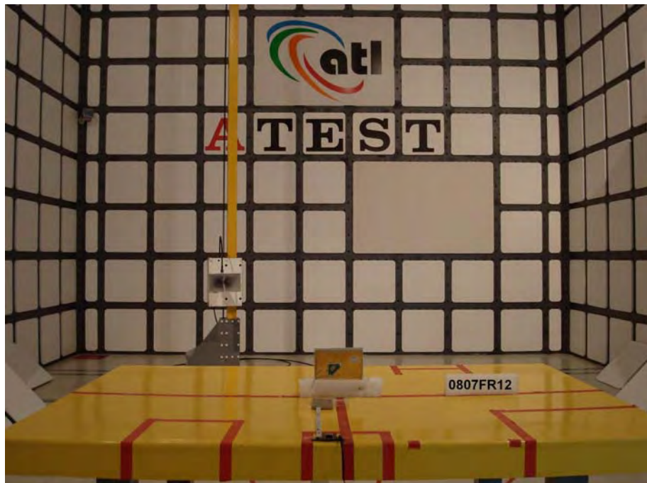
Figure 19. Rear View of the Test Configuration _ EUT with Antenna (ANT-915CPS-C)
