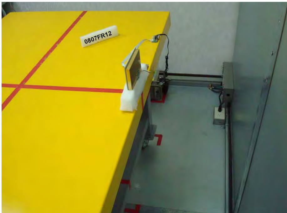
Figure 7. Rear View of the Test Configuration _ EUT with Antenna (ANT-915CPS-C)
