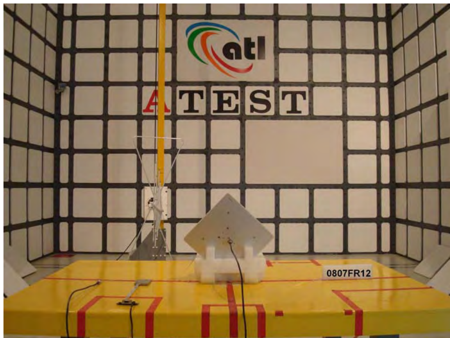
Figure 9. Rear View of the Test Configuration _ EUT with Antenna (ANT-915CPS-A)
