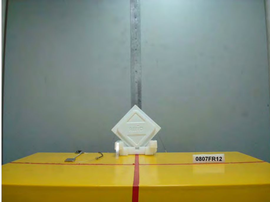
Figure 2. Front View of the Test Configuration _ EUT with Antenna (ANT-915CPS-A)
