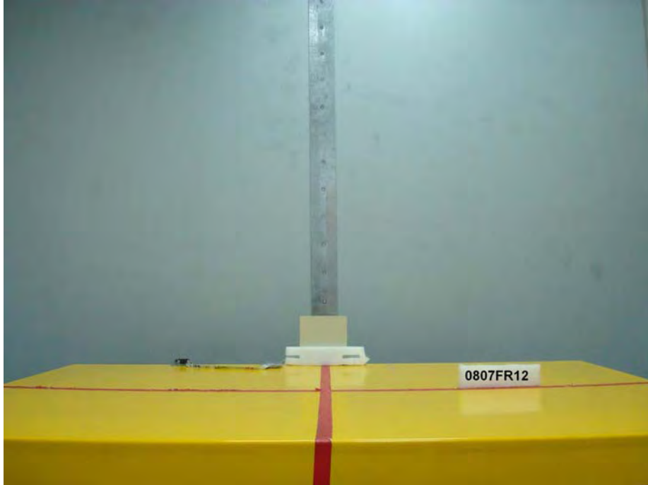
Figure 6. Front View of the Test Configuration _ EUT with Antenna (ANT-915CPS-C)
