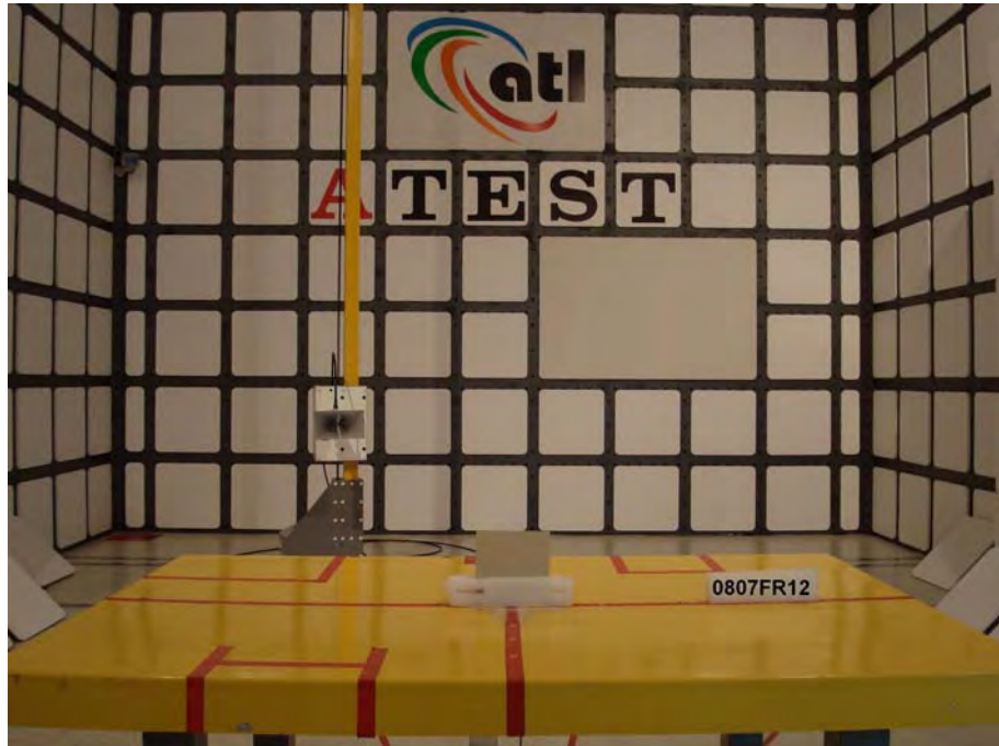
Figure 18. Front View of the Test Configuration _ EUT with Antenna (ANT-915CPS-C)
