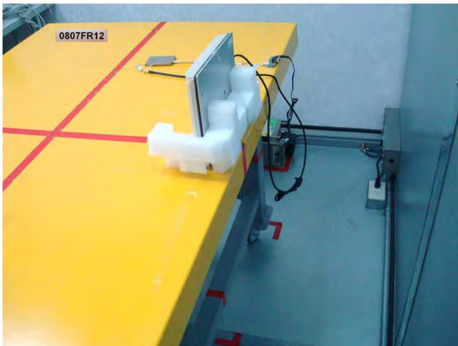
Figure 5. Rear View of the Test Configuration _ EUT with Antenna (ANT-2010CP)
