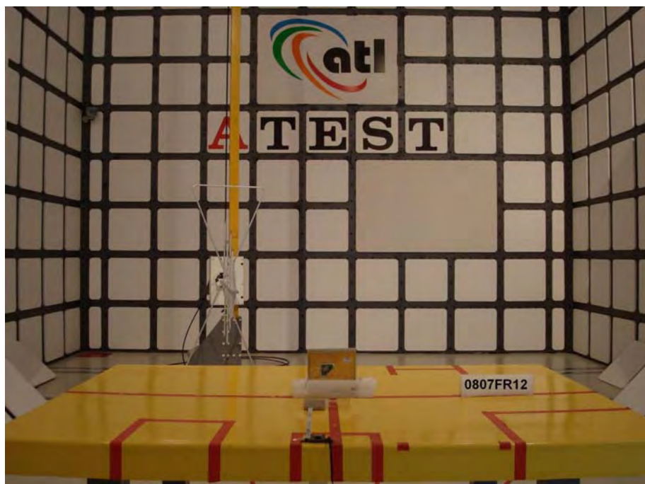
Figure 17. Rear View of the Test Configuration _ EUT with Antenna (ANT-915CPS-C)
