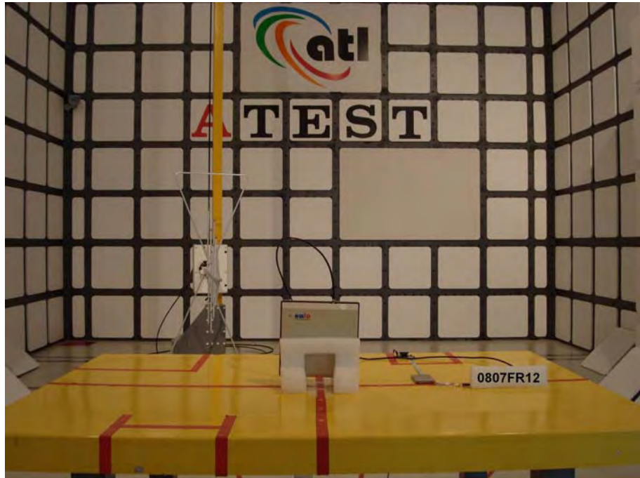
Figure 12. Front View of the Test Configuration _ EUT with Antenna (ANT-2010CP)
