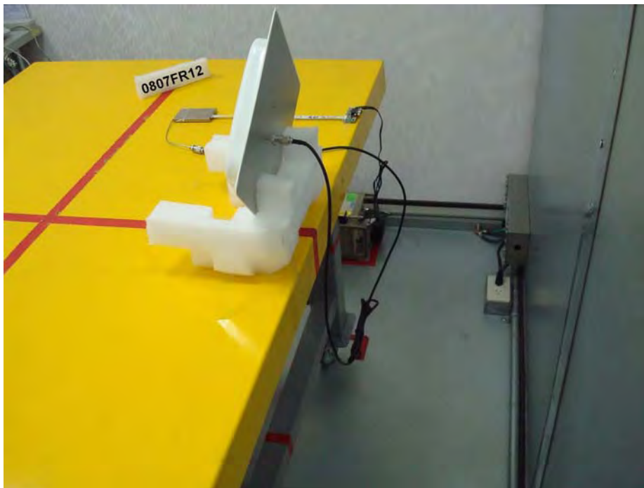
Figure 3. Rear View of the Test Configuration _ EUT with Antenna (ANT-915CPS-A)
