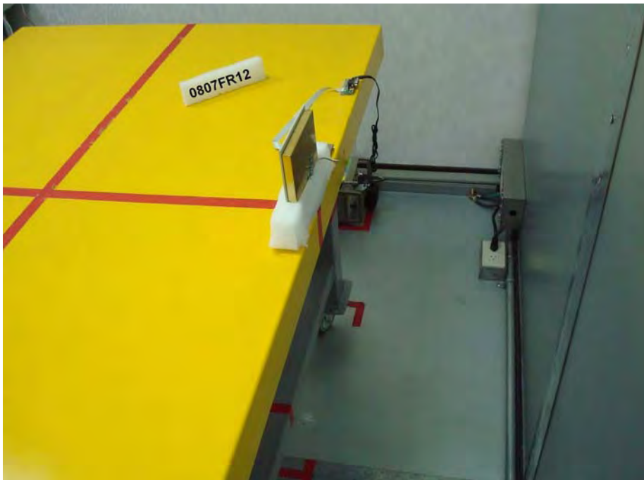
Rear View of the Test Configuration _ EUT with Antenna (ANT-915CPS)
