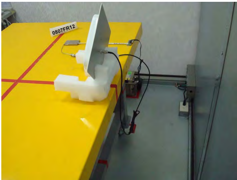
Rear View of the Test Configuration _ EUT with Antenna (ANT-915CPS-A)
