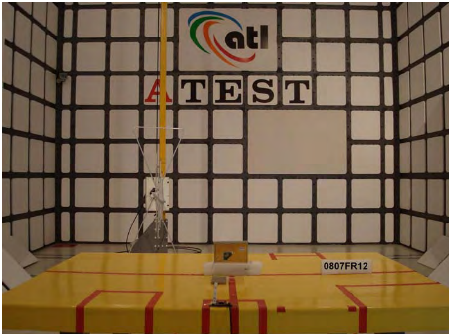
Rear View of the Test Configuration _ EUT with Antenna (ANT-915CPS-C)
