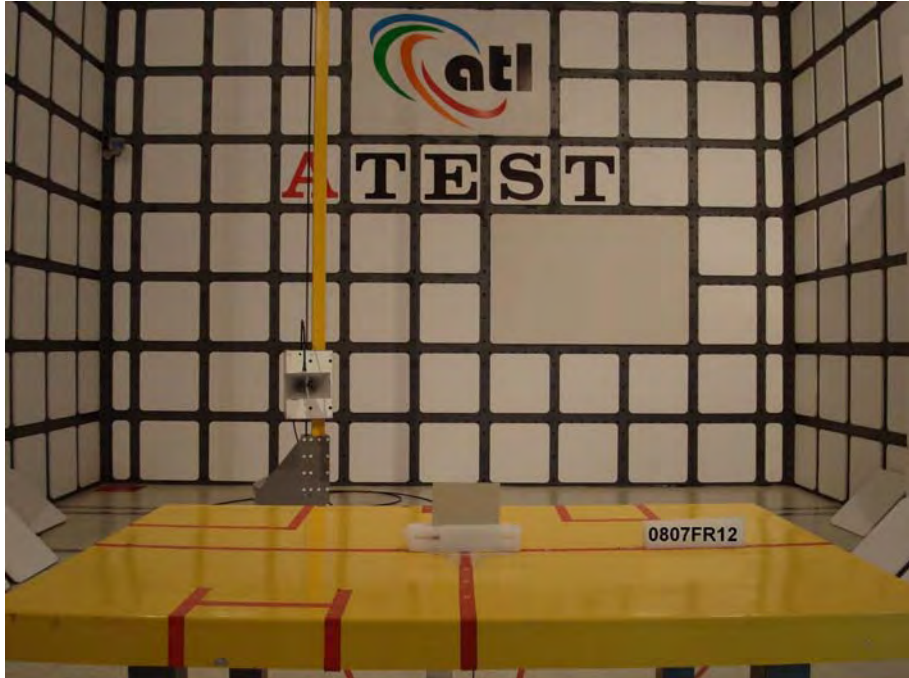
Front View of the Test Configuration _ EUT with Antenna (ANT-915CPS-C)
