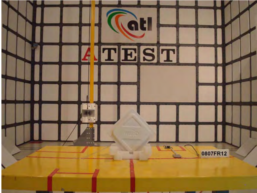
Front View of the Test Configuration _ EUT with Antenna (ANT-915CPS-A)
