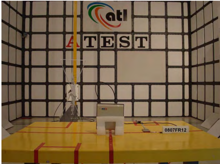
Front View of the Test Configuration _ EUT with Antenna (ANT-2010CP)
