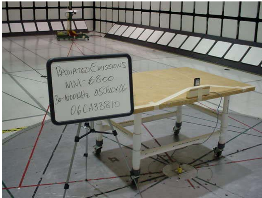
Radiated Emissions Test Setup (30 – 1000MHz)
