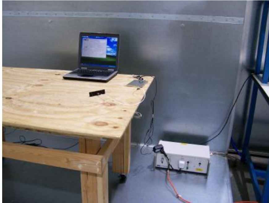
Conducted Emissions Voltage Setup
