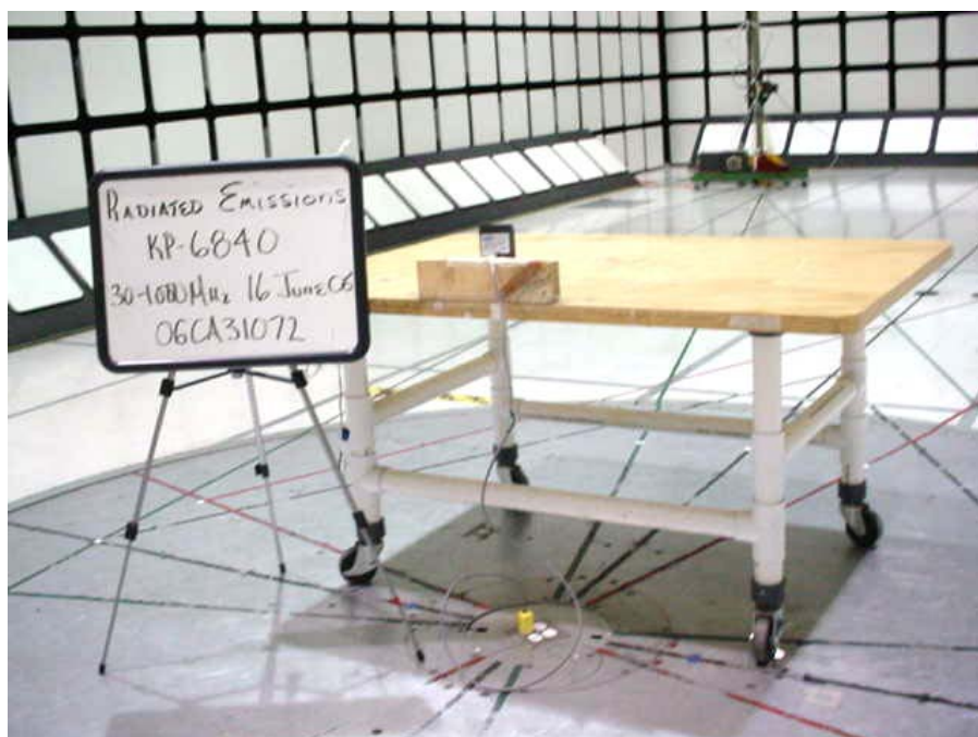
Radiated Emissions Test Setup (30 – 1000MHz)
