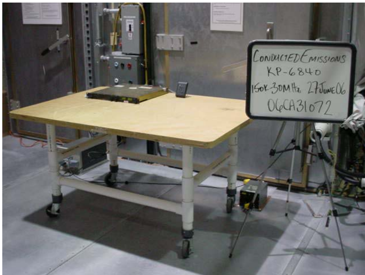
Conducted Emissions Test Setup (150kHz – 30MHz)
