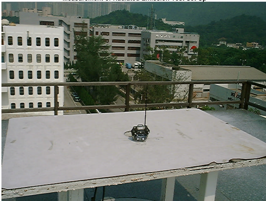
Measurement of Radiated Emission Test Set Up
