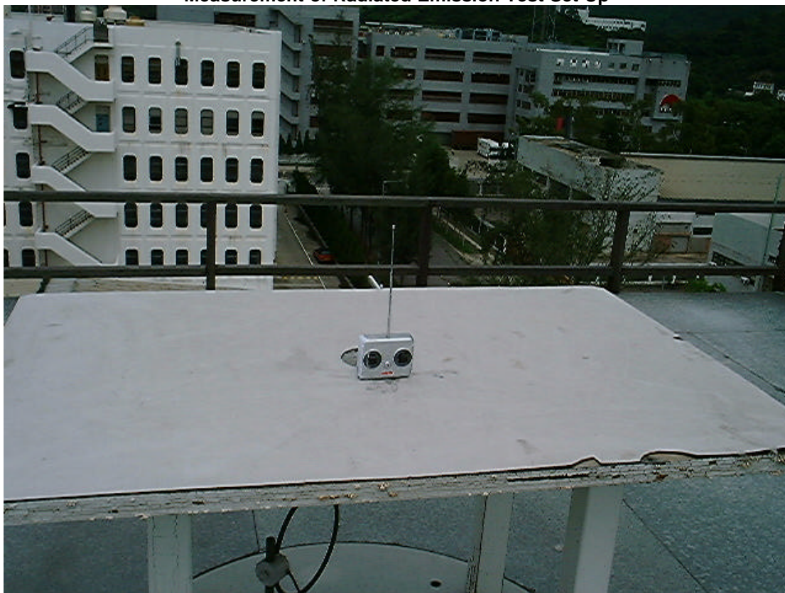
Measurement of Radiated Emission Test Set Up
