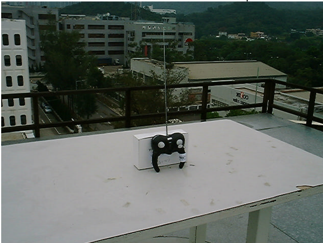
Measurement of Radiated Emission Test Set Up
