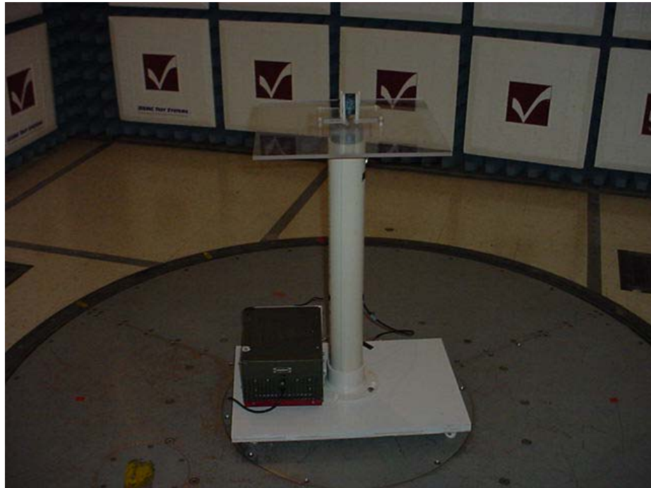
EUT Setup During Radiated Emission Testing
