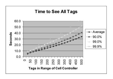
set and the very short 2.3 millisecond Tag signals minimize the number of Tag collisions. There is a possibility that Tag reads will be lost due to "collisions", particularly if there are large numbers of Tags in range of a given Cell Controller.
