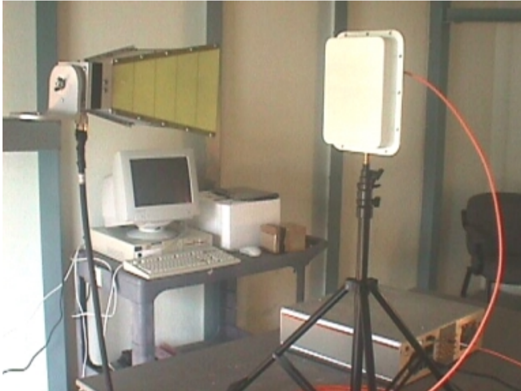
Harmonic Radiated Emissions 4-18GHz
