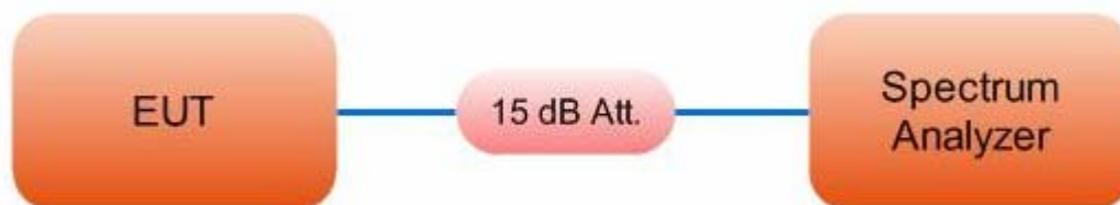
Figure 3. Occupied Bandwidth (Emission Mask) Test Setup
