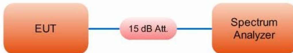
Figure 2. RF Power Output Test Setup
