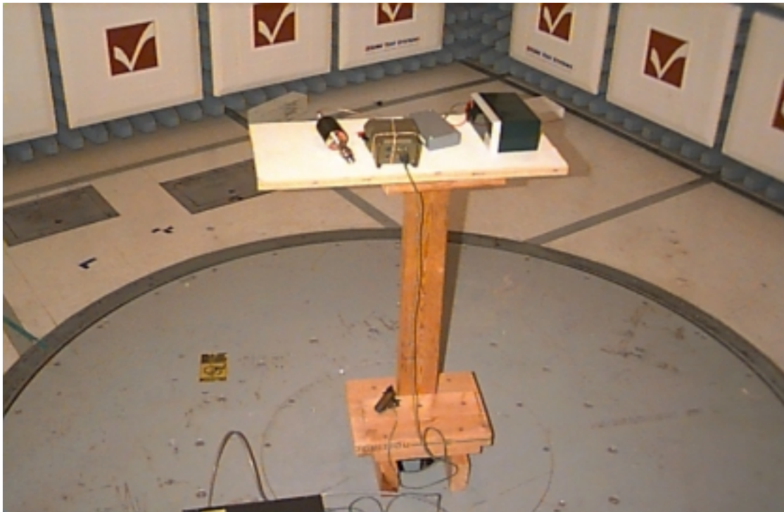
View of the EMIDS MMCT surveillance transmitter while performing Radiated Emissions Testing
