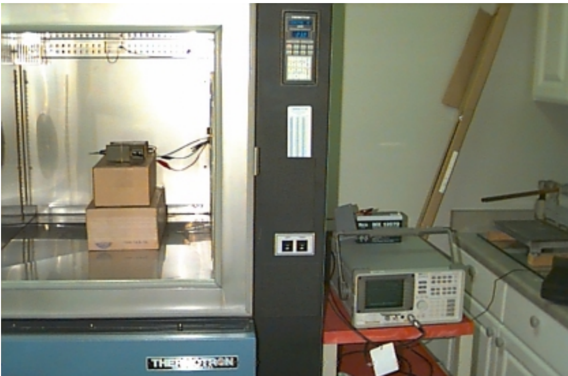
View of the EMIDS MMCT surveillance transmitter while performing temperature/stability Testing
