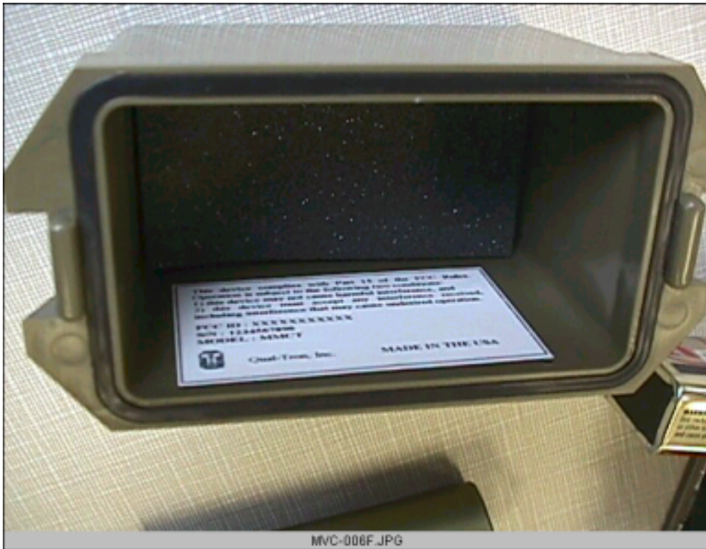
Qual-Tron - FCC ID Label installed inside of Battery Cover
