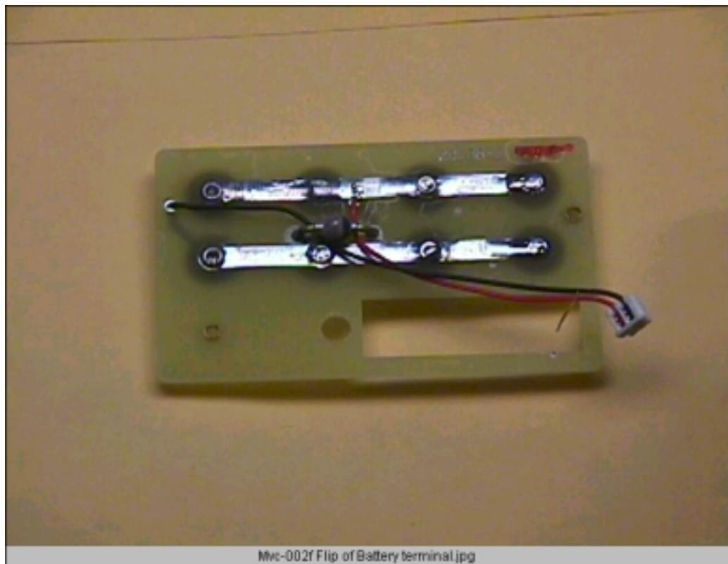
**Qual-Tron: Battery Terminal Board, Transmitter, Foil Side**
