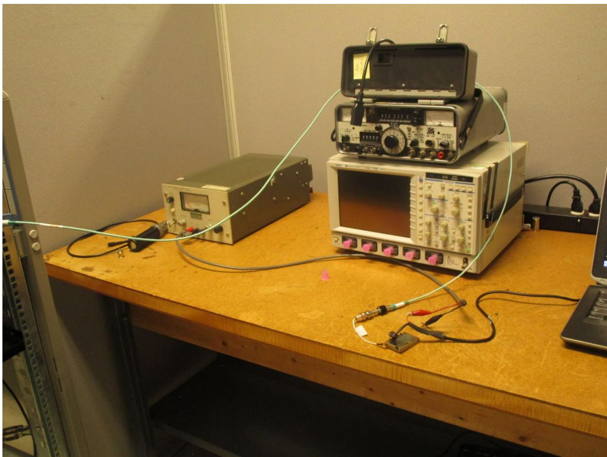
Frequency Stability Testing, Table Setup
