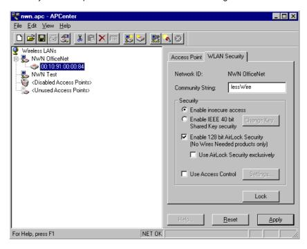
The tree structure on the left of the window shows a list of WLANs (Wireless LANs) and the Access Points that are part of each WLAN. The sample image above shows a single Access Point with hardware address 00:10:91:00:00:84 that is assigned to the WLAN named "NWN OfficeNet". The icons indicate the status of the WLANs and their associated Access Points.
