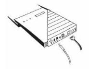
If all goes well, the rightmost LED (power) is green and the leftmost (WLAN) and middle (wired network) LEDs flash whenever there is traffic on the respective networks which is at least ten times per second for the wireless LAN because of so-called 'beacons'.
