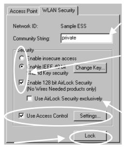
Use this button to lock the settings of the Access Points (almost) permanently
