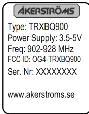
Figure 4. Label for the radio module
