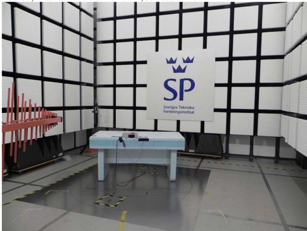
Picture 9, Antenna: Wire antenna 40 mm, 30-1000 MHz:
