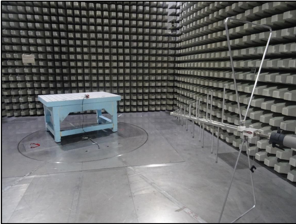
Photo 3 Radiated Test Setup from 30 MHz to 1 GHz
