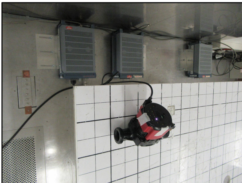
Photo 7 AC Conducted Test Setup
