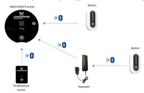
Figure 1 – Block diagram of the HWR-D system
