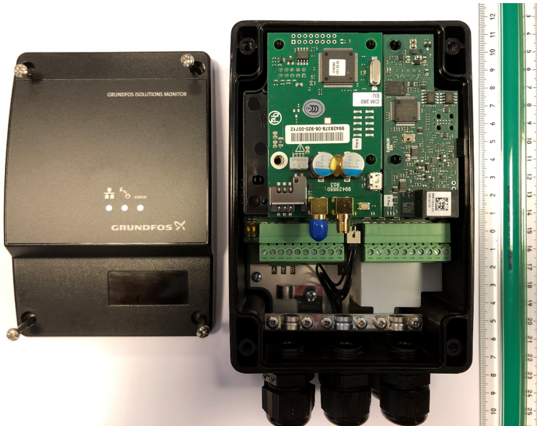
Inside view with enclosure removed
