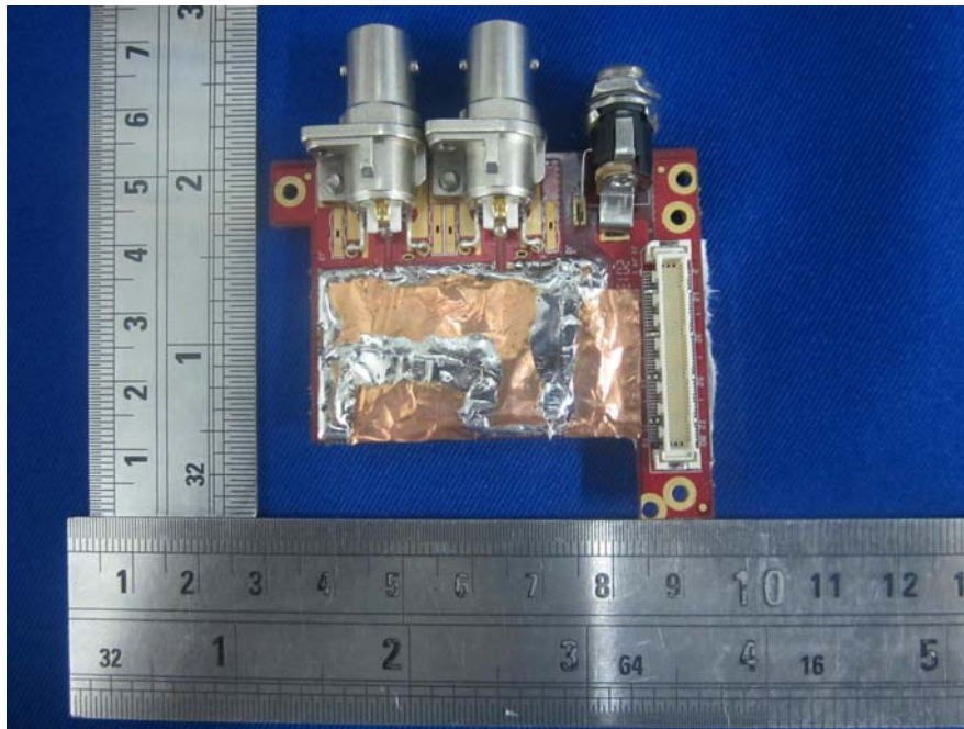
EUT – Sub Board Top With Copper Foil View
