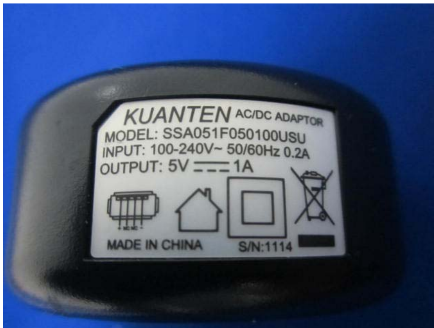
EUT – Adapter Label View
