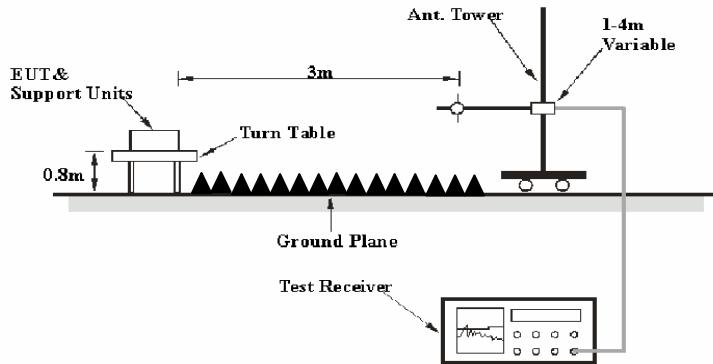
The radiated emission tests were performed in the 3 meters, using the setup accordance with the ANSI C63.4-2009. The specification used was the FCC 15.209, and FCC 15.407 limits.
