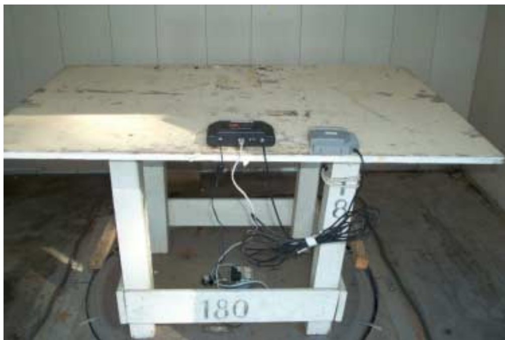
Typical Hosting I: Base Unit-Position X w/ Patch Antenna
